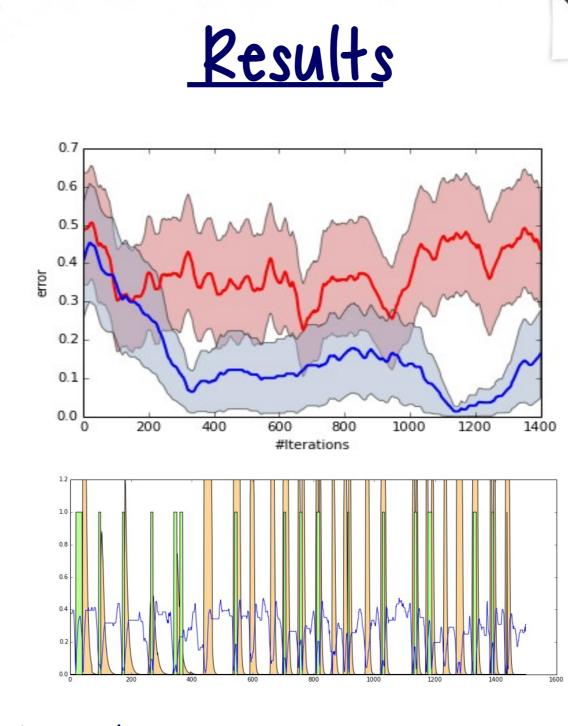
Errors decrease with time in the adaptive controller but not in the reactive. Top: mean and standard error of feedback received in ten independent experiments, for the adaptive (blue) and reactive (red) architectures. Bottom: boundary perception (blue), human feedback (green) and anticipated feedback (orange) learned from experience by the cerebellar model.
